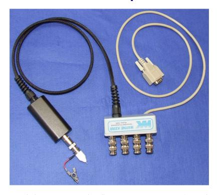
The 1J1025 Grounded Component Probe allows Wayne Kerr 6500 series analyzers to make ground referenced impedance measurements between 1 kHz and 120 MHz.
